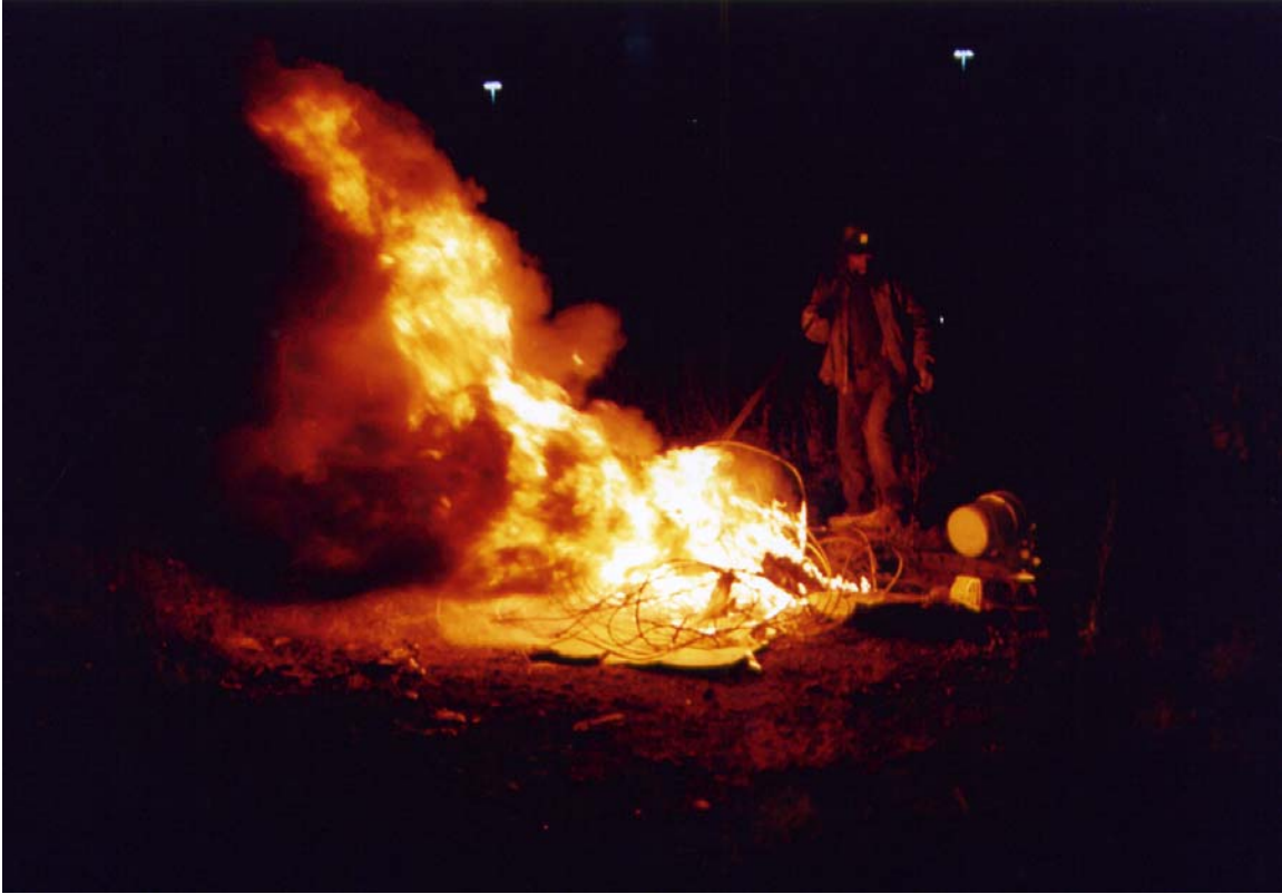
Scrapper "Country" burning the plastic coating off of copper cable.
